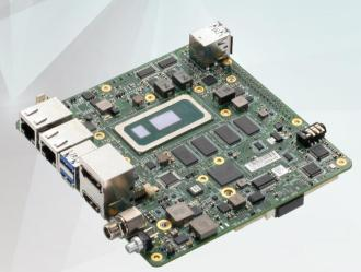
The UP Xtreme brings industrial grade features to the UP line of products, such as 12~60V wide voltage power input, two RS232/422/485 10-pin headers, and time sensitive networking (TSN) to facilitate communication in a connected factory. The UP Xtreme is also built to perform in temperatures ranging from 0°C up to 60°C.
